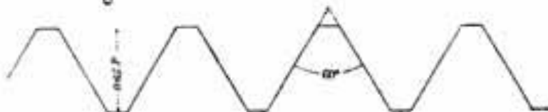
Fig. IV. Form of Thread proposed by Mr. Sellers.
