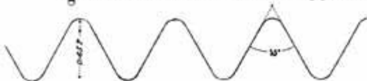
Fig. III. Form of Thread introduced Mr. Whitworth.
